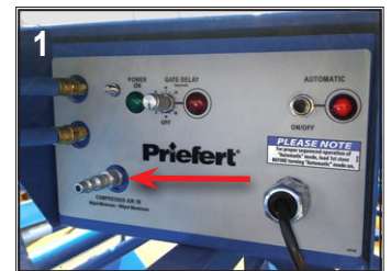
DIAGRAM 1 - Connect Air Supply (Male, 1/4" NPT Quick-Connect Shown)
