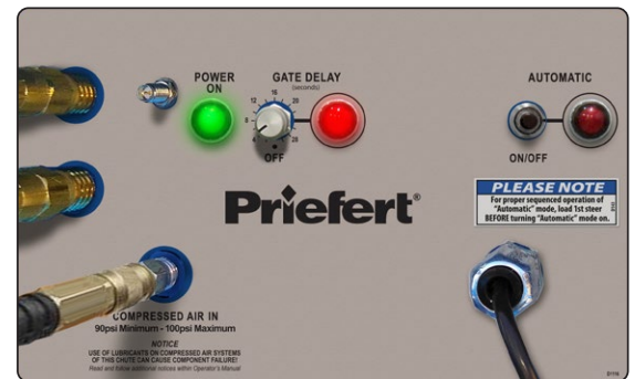
GATE DELAY “ON” & set to 4 sec.
