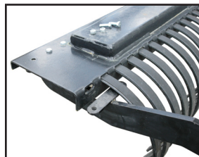
Figure 2 - Insert Bolt through wheel bracket
