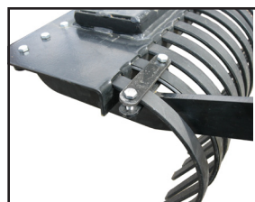
Figure 3 - Reinsert tine and bolt bracket
