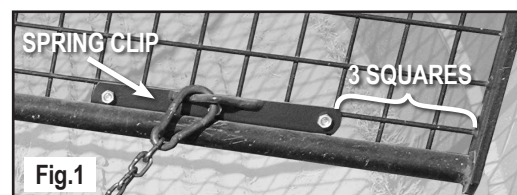
HW Drag Chain Plate & Backing Plate Assembly
