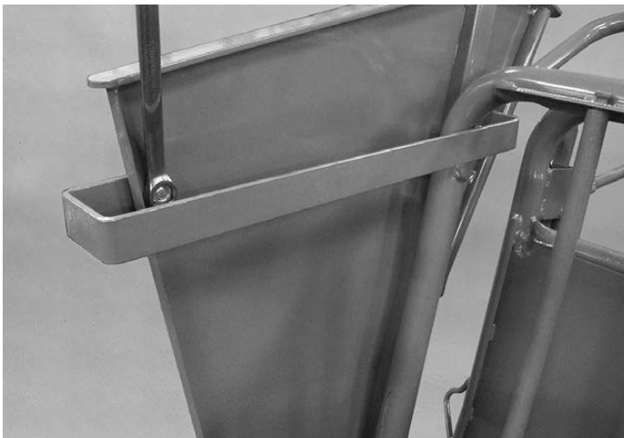
Figure 2-3 Remove Headgate Guide
