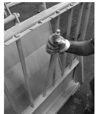
Figure 1-8 Side Bar Removal
