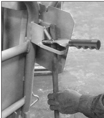
Figure 2-2 Remove Slip Rod
